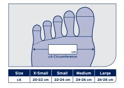
\* The mean compression for an average foot size with the related measurements.
