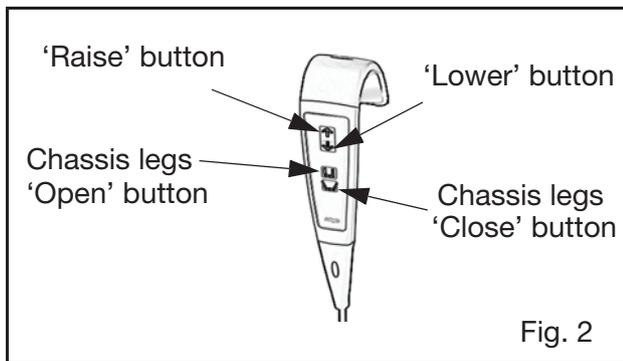
If pressure is released during any function, powered motion will stop immediately. Do not drop the handset into water, e.g. bath.
