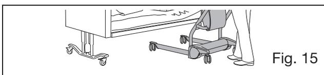
Only when the resident's body weight is fully supported by the bed, may the sling connection loops be detached and while still in sitting position, detach the sling from the hooks before reclining the resident to the bed.
