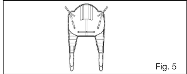
Place the sling around the resident so that the bottom of the back support area reaches the bottom of the resident’s spine (it is not necessary to pull the sling under the resident). Ensure the head support area is behind the head (See Fig. 5).
