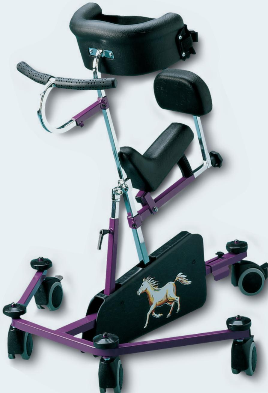
The Pony has a frame shaped like an arrow with five castors. A central bar holds the chest support and the seat with pelvic support. The bar can be tilted forwards to stimulate walking. Between the legs is a plate to avoid scissoring. The Pony is for indoor use.
