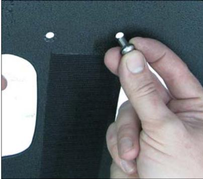
With cushion removed, insert M6x10mm button head with one serrated washer through the inside of the backrest.
