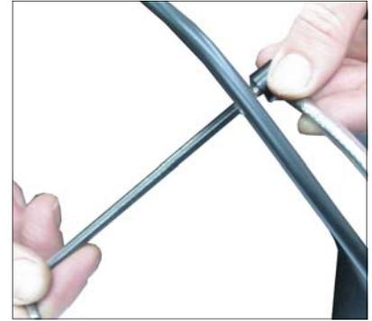
With the cable fully inserted into the cable end piece, thread bolt into cable end.
