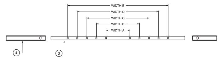
Place the combined Items 4 and 3 approximately 6 to 12 inches above the crease between the head and lower portion of the bed. Attach an Item 2 to Item 4 using Items 7 and 8, but do not fully tighten. Place the first Item 2 over the side of the bed that raises the head up and down.
