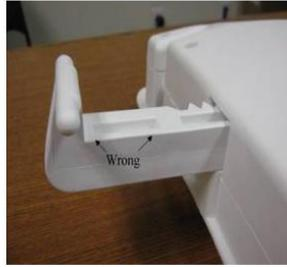
19. If the back is to be removed for easy transportation the lifting rod must be fully retracted. If it is not when it is separated use the hand control to fully retract the lifting rod.
