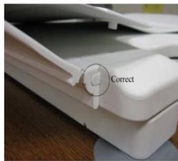
15. Before the locking buttons on the seat cover can be engaged the wings of the seat must be pushed forward. If they are not the locking buttons will not line up with their receiving holes.
