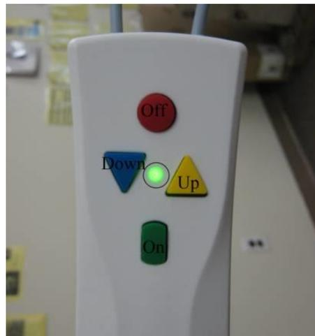
18. The unit is ready to be used. Turn the unit on by pushing the green button on the hand control. To bring the unit up, push the yellow button and to bring the unit down, push the blue button. Push the red button to turn off the unit. If the unit is left on for more then 30 minutes it will automatically shut off.
