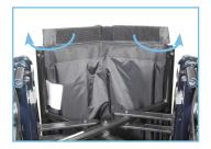
2. Pull outward on hook and loop fastener strips to free them from underside of seat.
