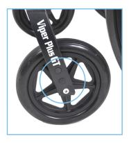
The 3 position front caster can be adjusted for positioning with the rear wheel. To adjust the front caster, loosen the bolt (outside of the caster) with an allen wrench (included). Remove the bolt and axle and place into the desired position. After the axle is placed in the new position, turn the allen screw clockwise to tighten.
