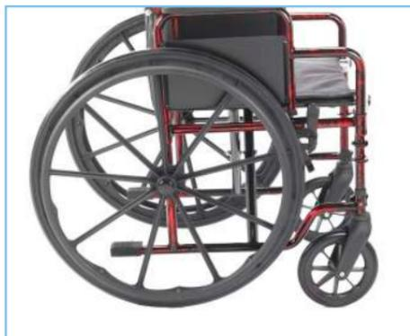
To remove wheel, depress spring loaded button and slide wheel out from axle port.
