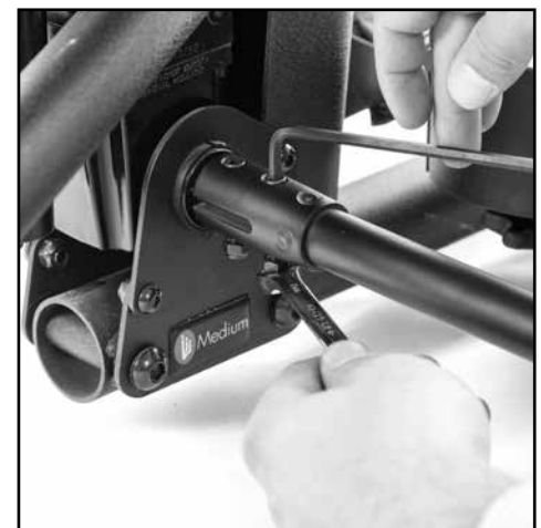
24. Place pump handle back onto the pump. Insert bolts and nuts and tighten securely.
