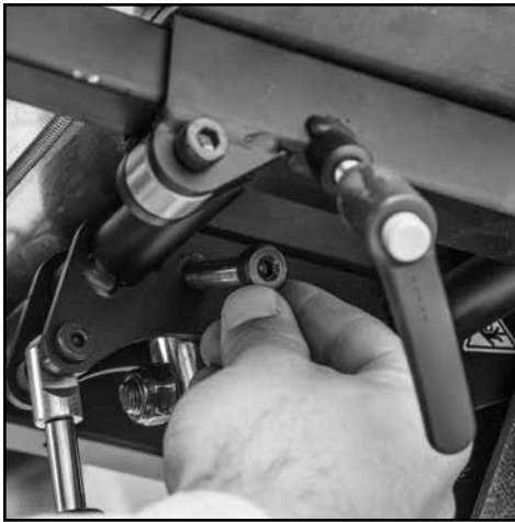
19. Line up holes on the seat and pump. Insert bolt and place nut onto bolt.
