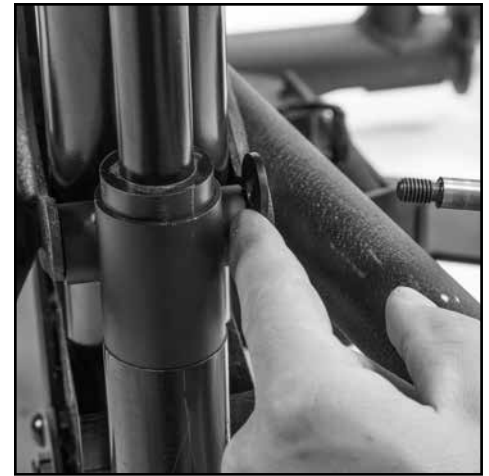
21. If you do not have the Supine option skip to step 24. Place right side washer between the brackets on the dampener cylinder and insert bolt.
