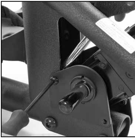
16. Use a 13mm wrench and hex wrench, insert the bolt and nut from the upper part of the pump bracket. Tighten securely.
