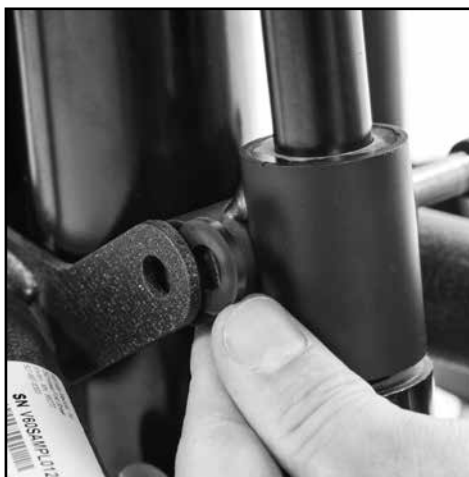
22. Place left side washer between the brackets on the dampener cylinder and insert bolt.
