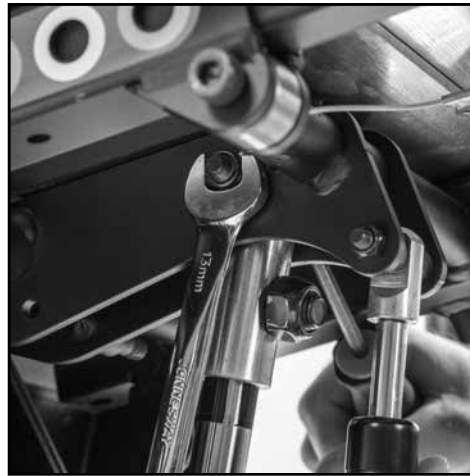
20. Use a 13mm wrench and hex wrench to tighten the nut and bolt for the pump.
