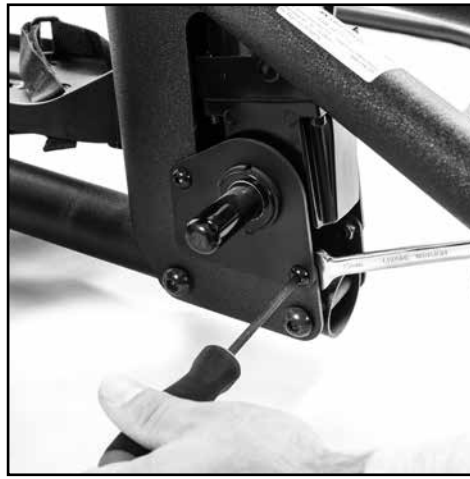
17. Use a 13mm wrench and hex wrench, insert the bolt and nut from the lower part of the pump bracket. Tighten securely.
