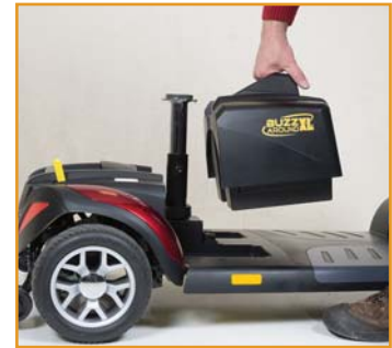
Step 2: Pull out the battery pack!
