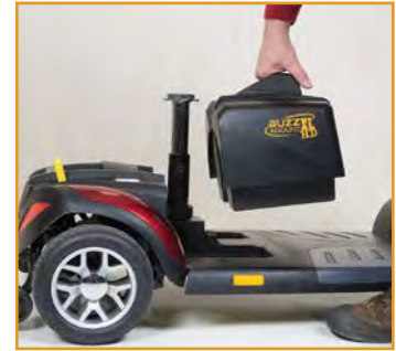
Step 2: Pull out the battery pack!
