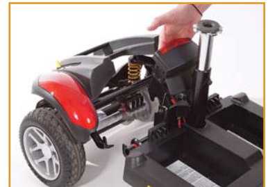
Step 4: Pull forward on the drivetrain release lever to separate the front and rear frame sections!
