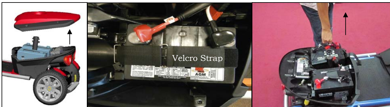
Figure 13. Removing the Batteries
