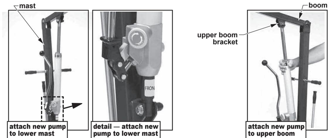
1. Attach the bottom of the new hydraulic pump to the lower mast bracket with the pressure knob and pump lever toward the bottom of the pump, as shown at above left, and the “**FRONT**” label toward you, as shown at above center. Use a hex bolt, washers, and hex nut to secure pump to mast. Use two  $\frac{9}{16}$ ” wrenches to tighten.
