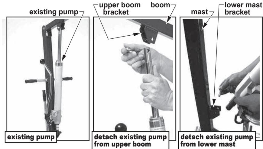
1. Follow the instructions in this section to remove the existing pump, shown at above left. If installing pump for the first time, proceed to **Installation of new pump** on next page.
