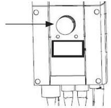
Grasp the handset, press the up button and run the lift arm all the way up. Then, press the down button and run the lift arm all the way down.
