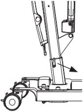
Place the mast in the base. There are three alternatives for adjusting the height of the mast. Secure the mast with the locking handle.
