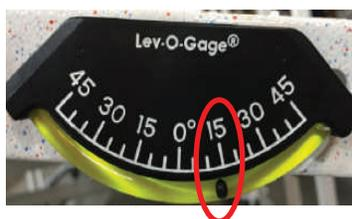
*The Tilt Indicator pictured above shows a Standard Crib crib with the foot/knee section raised to its maximum height position of approximately 15 degrees.*
