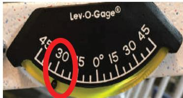
*The Tilt Indicator pictured above shows a crib with the head raised to its maximum height position of approximately 30 degrees.*
