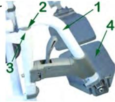
8. The foot plate height can be adjusted by loosening the footrest clamp (1), sliding the foot plate extension tube (2) up or down inside the foot rest hanger tube (3) and re-tightening the clamp.
