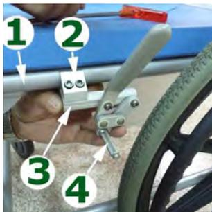
2) Position the knurled brake bar (4) horizontally in front of the tire and slide the entire assembly along the seat rail as needed until the distance from the front of the wheel lock mounting bar to the front of the seat rail is approximately 8.5 cm (3 3/8").
