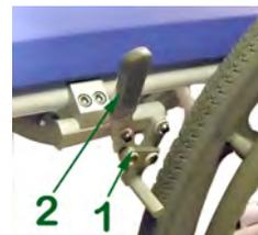
To engage the wheel locks (1) push the brake levers (2) forward until they lock. To release, pull the brake levers backwards.
