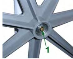
2. Holding the wheel by the spokes, once again push the quick release button (1) with your thumb and pass the portion of the axle protruding through the back of the wheel through the axle housing (2) until the axle protrudes all the way through (3).
