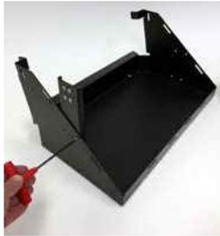
5) OPTIONAL: Install the "LTV Tower" on either side with of the rear tray with the supplied #8-32 x 3/8" screws (4). The "LTV Tower" is pre-drilled and threaded for the dovetail wall mount (not Included but pictured below).
