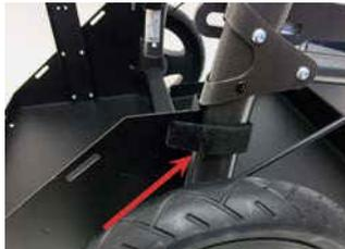
8) Loop the strap around the oval rear upright and below the round horizontal strut. Loop the strap thru the "D" ring and secure snugly back to itself with the velcro.
