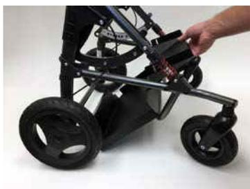
4) Pull the front of the tray up and over the front crossbar. Hook the back of the middle section over rear cross bar.
