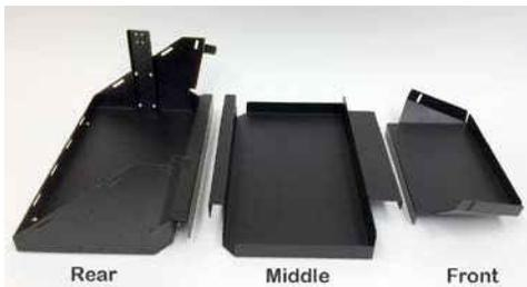
1) The respiratory equipment tray is three separate pieces that can be used in various combinations or as a complete system. The Middle portion hangs on the two chassis cross bars. The Front portion bolts onto the Middle portion with supplied #10-32 3/8" socket head cap screws. The Rear portion hangs on top of the Middle Portion across the same rear chassis crossbar and is additionally reinforced with supplied "D" ring straps for support.
