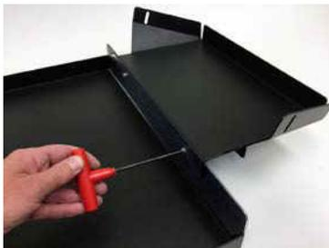
2) Place the Front tray on top of the wider edge of the Middle tray. The Front tray has two pre-drilled holes. The Middle Tray has two matching threaded inserts. Use the supplied #10-32 x 3/8" socket head cap screws and lock washers to bolt the two sections together. The front section of the tray will remain suspended between the two front casters. Slots in either "wing" are supplied for optional strap reinforcement as deemed necessary by the user.
