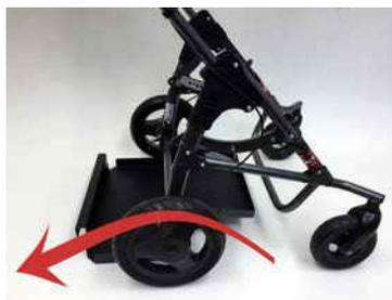
3) TILT OR REMOVE THE SEATING SYSTEM. The image to the left shows the chassis with the seating system removed for clarity. Place the tray on the ground behind the rear wheels. Roll the stroller backwards while lifting the rear cross bar over the front section of the tray.
