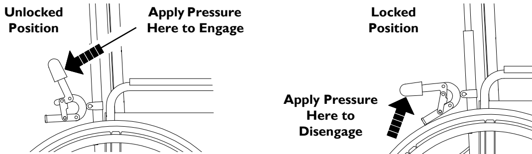
FIGURE 5 Using Attendant Operated Wheel Locks
