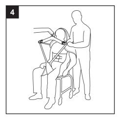
Position the head support around the back of the client's head. Attach the head support strap buckle and adjust the strap and buckle until the client's head is comfortably supported.
