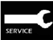
When it is time for a service, the service symbol will appear on the display. In addition, when the user handset is activated, the Smart Monitor will give an audible signal giving notice to users that a PM check is recommended (see recommended maintenance schedule later in this manual).
