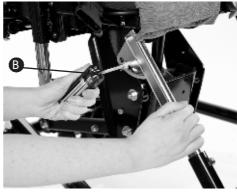
The footplate angle can also be adjusted for dorsiflexion and plantarflexion. To adjust for dorsiflexion, insert your Allen key in to the bolt below the footplate, directly in the centre, and turn right. To adjust for plantarflexion perform the same instructions but turn left.
