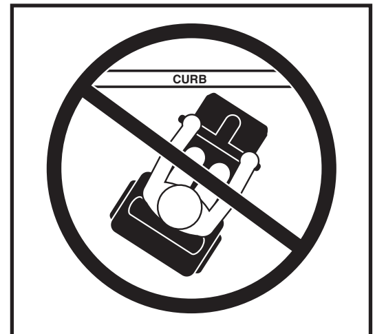
Figure 7. Incorrect Curb Approach
