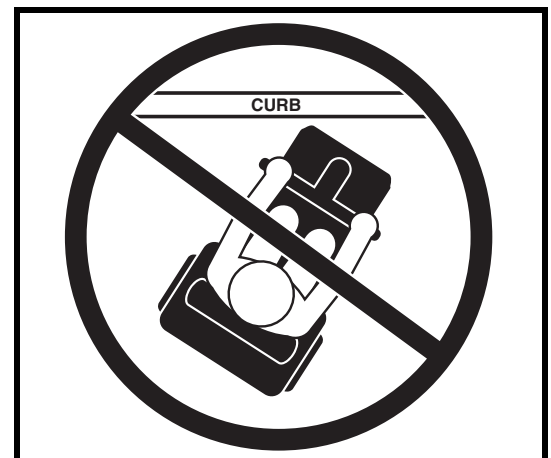
Figure 7. Incorrect Curb Approach
