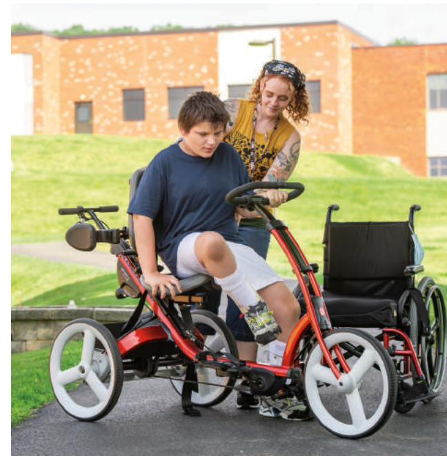
The laterals and handlebar swing away for easy transfers.
