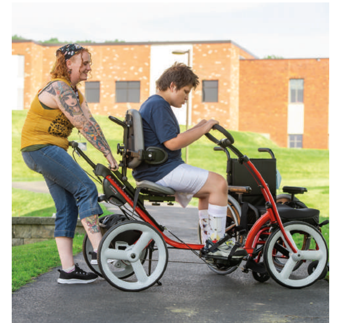
The seat glides up and down on a low-friction rail. This rider pushes with his feet to help his caregiver raise the seat.
