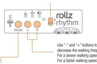
Use "-" and "+" buttons to increase or decrease the walking frequency in steps/min. For a slower walking speed, press "-". For a faster walking speed, press "+".
