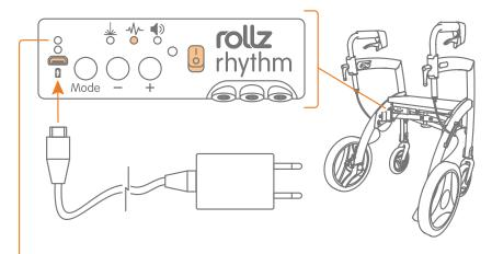
The module will display a red light while charging. When fully charged, this light will turn green. Charge the module only with an adapter of 5V and 1A.
