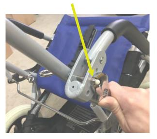
**Step Four:** Using an adjustable crescent or 10mm wrench, remove both adjustment nuts from either side of the chair.
