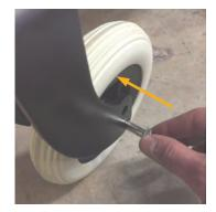
**Step Two:** Place the washer and nut on the bolt on the inside of the chair frame and use an adjustable crescent or 10mm wrench to tighten the bolt, securing the wheel.
