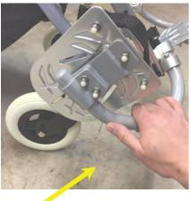
**Step Two:** On each foot plate, use an adjustable crescent or 10mm wrench to loosen the two depth adjustment nuts, pictured to the right.
