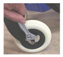
**Step Two:** Slide the bolt out of the fork and wheel. The wheel may now be removed.
