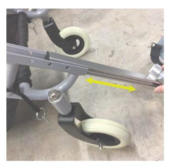
**Step Two:** Insert each foot plate rod into the grooved receiver tracks on each side of the chair.
