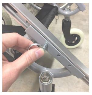
**Step Three:** Adjust each foot plate to the desired height. When in the desired location, secure each foot plate by inserting the locking pin into the corresponding hole on the receiver track.
