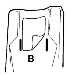
2> If Velcro® hook and loop fasteners are exhausted and have lost their holding power, a new Velcro® patch of larger dimensions may be adhered on top of the old Velcro®. Adhesive may be used if a stronger bond is required. (C)
