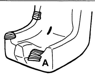
3> Cover the damaged area with the colored press patches in an overlapping sequence as shown.(A) Peeling off the paper backing is easier if you slightly tear an edge of the patch far enough to get a fingernail under the paper. Apply the patches as you would adhesive bandages.
